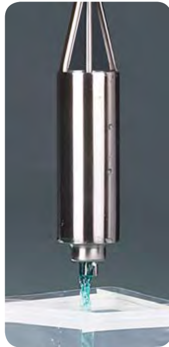
The valve is opened with the thumb to empty the sample.
