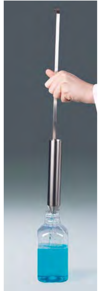
The valve is opened by attaching the sample container to empty the sample.
