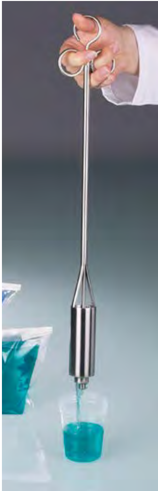
The valve is opened with the thumb to empty the sample.
